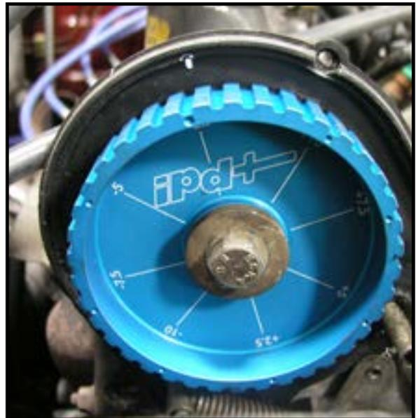
photo #2 - Outer timing mark lines up with timing mark on back cover. Please note that on early models this mark is cast into the cam cover.
