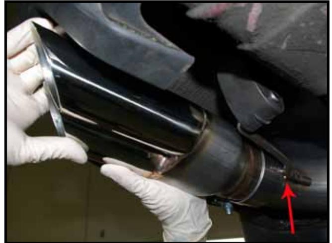
Exhaust tip is fully seated against rear exhaust hanger.
