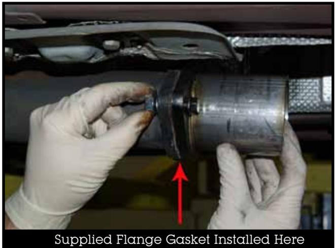
Supplied Flange Gasket Installed Here
