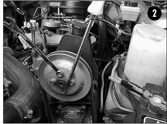
Wedging a screwdriver between the pump nose and mounting bolts will ease pulley removal and installation.
