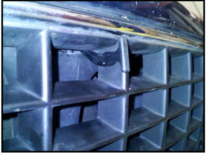
**4** Note the existing spring in the factory location as shown and remove it from the release assembly.
