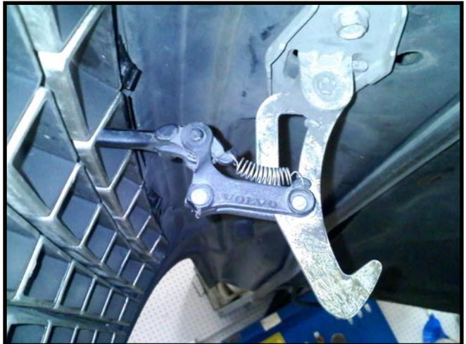
**5** Modify the spring using a small pair of needle nose pliers so that it resembles the spring in the picture.
