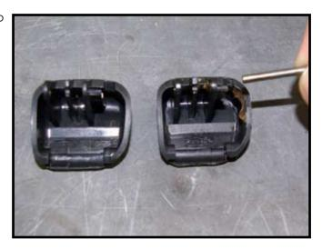
8 Now snap the release knob back into the housing as shown.
