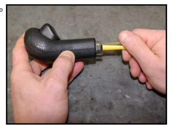
With the shift knob release button exposed, use the screw driver to pull the button away from the housing and expose the internal spring.
