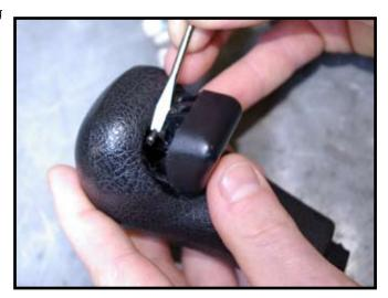
Now remove the release button from the housing by pulling it out and away from the shift knob.
