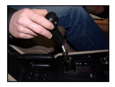
Reposition the shift selection boot back onto the shift knob.
