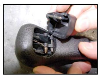
Reposition the internal spring back onto the release knob using a small flat blade screwdriver.
