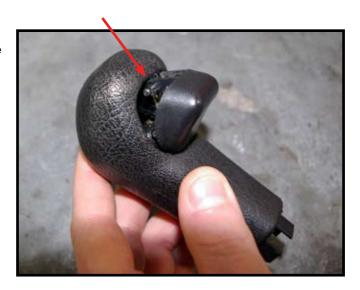
4 Use the screw driver to release the internal spring from the release button.
