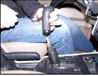
With the shift knob removed use a small flat blade screw driver to push the release arm from within the shift knob housing.
