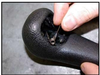
7 Transfer the steel rod from the old release knob to the new release knob.
