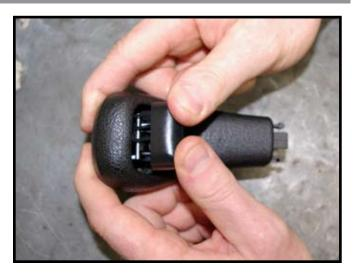
Install the shift knob back onto the shift selector, use moderate force to reattach the unit by pressing downward with a sharp 'smack' with your palm.
