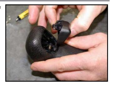
6 Note the original orientation of the original internal spring and replace it with the new included.
