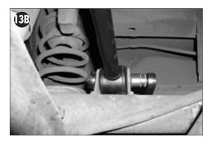
Press in the new poly bushings using a vise. Once both bushings are installed, apply a moderate amount of the supplied grease to the inside of the bushing and press the center sleeve into place.
