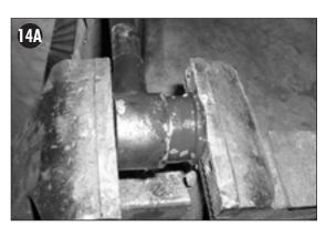
Reinstall the first torque rod and proceed to the next one. Repeat the same procedure.
