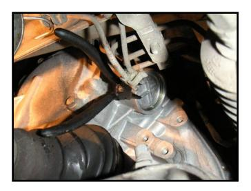
Use pliers to wiggle the plug free of the transmission case, a twisting motion will work best.
