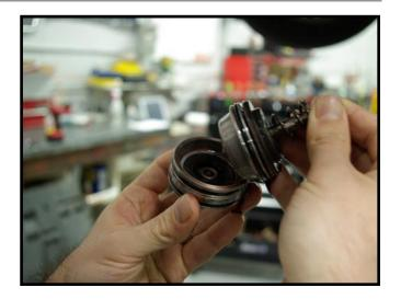
Insert the B4 piston and cover into the transmission and push them in far enough to allow the snap ring to be re-inserted.
