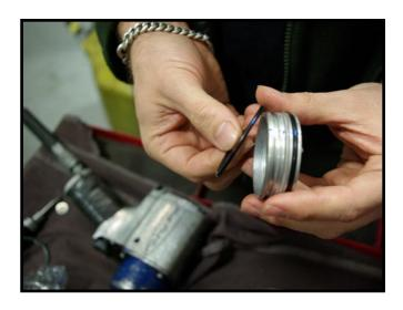
8 Use the remaining O'ring from the kit to replace the O'ring on the B4 piston.
