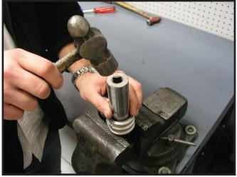
The bushing has a plastic outer sleeve and should only require low to moderate force to remove it from the bracket.
