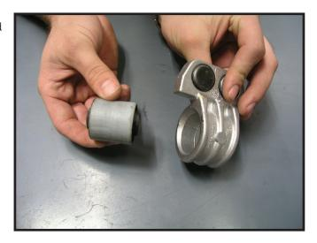
Install one half of the new polyurethane bushing into the bracket. (Some mounts may have a slight eliptical shape to them. This is normal. A moderate amount of pressure may be needed to conform the bushing to that shape.)
