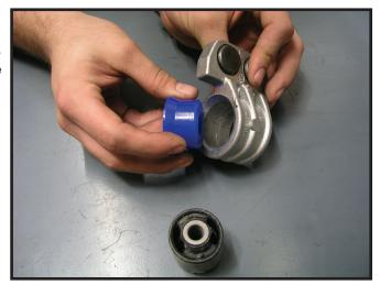
Install the other half of the new polyurethane bushing into the bracket
