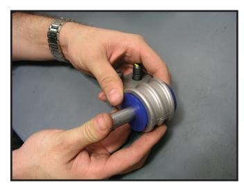
Reattach the bracket to the rest of the transmission mount and insert the bolt and nut that was previously removed.
