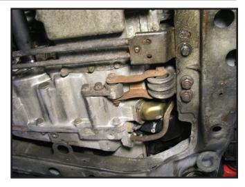
Remove the two 14mm bolts as shown.
