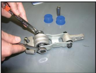
6 Seperate the bracket from the rest of the mount.
