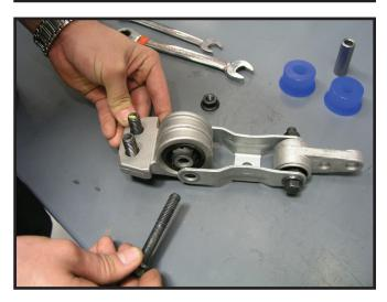
Use a socket or piece of steel that is approx. 1.3 inches in diameter.
