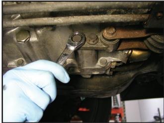
3 Remove the two 18mm nuts as shown.
