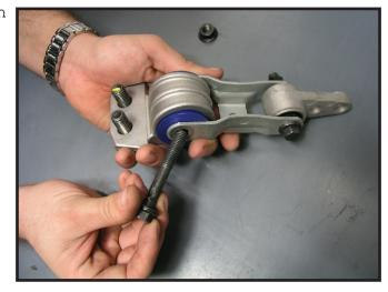
Note the orientation of the bracket to the mount and be sure assemble it correctly as shown. Tighten the bolt and nut to 20 ft lbs.
