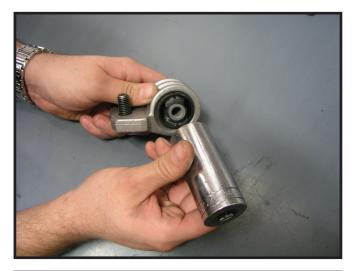
8 Set the bracket in a vise and use a hammer to tap the bushing out of the bracket.
