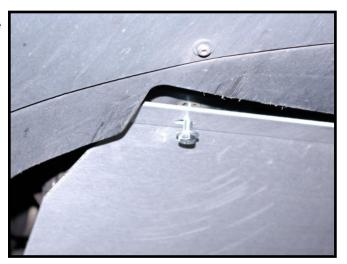
Move to the rear of the skid plate and using the included 12mm bolts and washers fasten the rear of the skid plate to the vehicle's via the existing threaded mounting holes. \*Be Advised, the washers should be placed one on each bolt as well as one between the skid plate and the vehicle chassis so that the skid plate does not rest directly against the subframe, this is done to reduce the possibility of noise.
