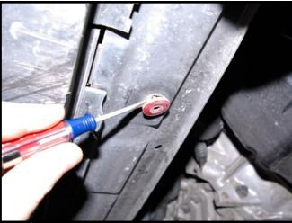
Place the two 8mm nuts on the top of the radiator support where the plastic nuts were previously.
