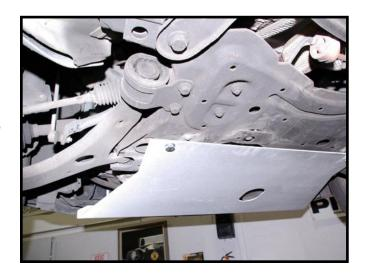
Now, tighten the 8mm bolts to 20 ft/lbs and the 10mm bolts to 30 ft/lbs
