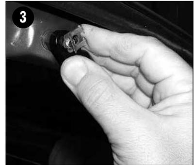
**4** The hinges are held to the body by 2 bolts (13mm) and the hinge is attached to the tailgate with a 13mm bolt and a large Phillips head screw. The bolts are screwed directly into the base of the hinge. The large Phillips screw is accessed through a small hole in the gate about 3" away from the hinge. Loosen all the hinge fasteners about one full turn, but do not remove yet.
