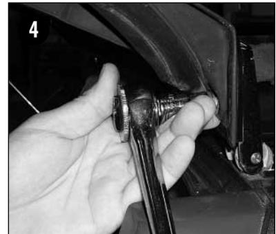
**5** Before removing the gate, prepare an area where the gate can lay without scratching the paint. Close the gate and from the inside, unbolt the tailgate hinges from the body, pull the wires through the roof and, with the aid of an assistant, carefully remove the gate (you will need to press the release latch to open the gate as it is lifted away from the body).
