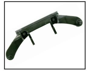
The hinge in this picture may not appear identical to your hinge and gas door, but similar techniques are used for the install of each part. Check the replacement part carefully to assure it is the correct component for your car.
