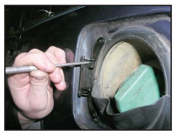
Gently flex the door into position and reseat the spring as original. Do not force the door but ease it closed to check for interference and proper hinge function.
