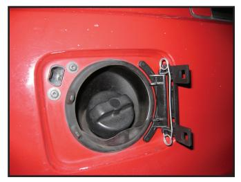
Next, attach the gas door using the factory screws by hand, align the door to the body opening, then tighten the screws properly.
