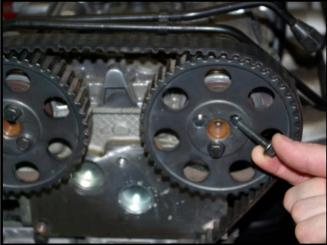
Install the cam timing tool as shown with the graduation marks that are labeled "intake" aligned to the factory mark on the intake cam gear and reinstall the two 10mm bolts, screw the bolts in to take up the slack but do not tighten.
