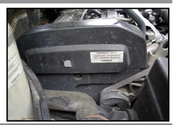
2 Using a 30mm socket rotate the engine clockwise at the crank pulley nut until the factory cam gear marks line up with the corresponding top engine cover marks.
