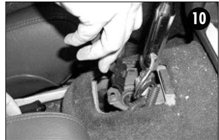
**10** Using snap ring pliers remove snap ring at the base of the shift lever that retains the shifter. Depending on orientation of snap ring you may need to unbolt reverse lock out plate. Be sure to scribe a mark to aid in reinstallation and adjustment of the reverse lockout plate.
