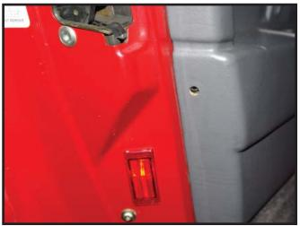
9 Lift the door panel up and away from the door and disconnect the speaker wires.
