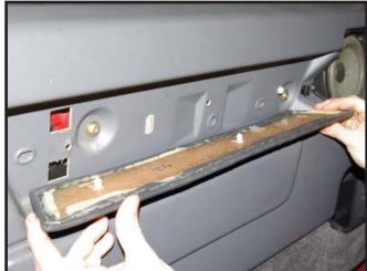
5 Remove the two torx 30 fasteners from the door panel.
