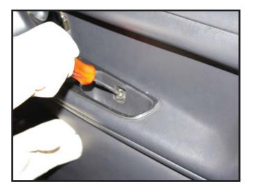
Loosen the door panel from the door frame going around the perimeter of the panel using an interior tool as shown.
