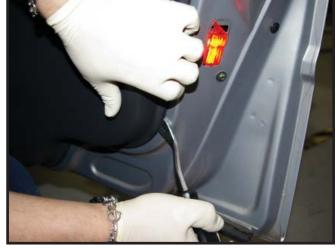
8 Lift the door panel up and away from the door frame and disconnect the inner door handle cable by gently pulling it away from the handle mechanism and disconnect the window switch wire harness.
