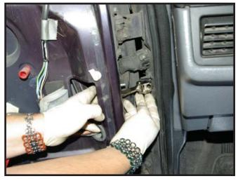
Remove the two 10mm nuts holding the door check strap to the door frame.
