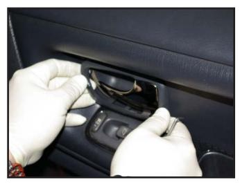
4 Remove the outer mirror cover by gently prying it away from the door frame.
