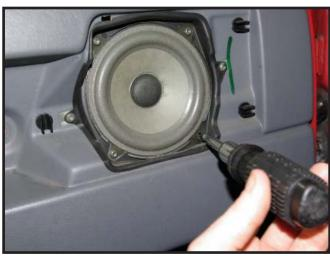
7 Remove the four torx 25 screws at the base of the door panel.
