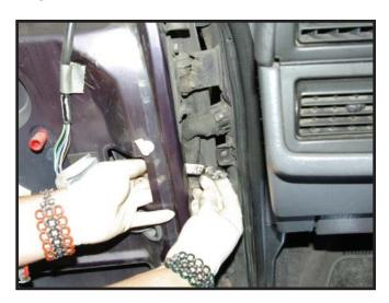
To remove the door check strap from the door frame you will need to rotate it so it can clear the internal components in the door.
