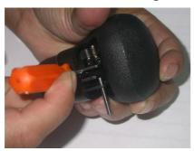
3).Release the spring by using the needle –nose pliers. (See diagram 3)
