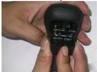
2). Insert pin into the push button upper hole. The pin must go through
