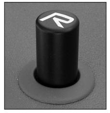
Thank you for purchasing ipd billet aluminum door lock pins. Our pins feature a nice, smooth, durable satin finish that comes from tumbling the machined parts in a mild abrasive media prior to anodizing. All pins are anodized. Even the brushed aluminum versions are clear anodized so they will not stain scratch or need polishing in normal use. The R logos are laser etched into the aluminum for a lifetime of service.
