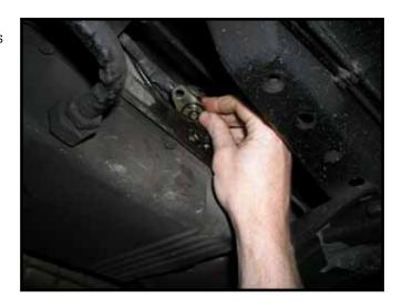
Place the new ring in the groove on the bypass plate and set on the transmission flange in the same position the solenoid was removed. If the bolts are started and the outer edges do not align, it may be installed backwards.
