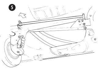
Angle tightening means to tighten the bolt to the specified torque and then tighten beyond to the specified degrees.
