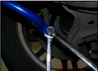
The second endlink style is for S80, XC90, S60, and V70 2001-2007 and uses a 5mm allen wrench and 19mm end wrench to tighten the nut to the stud.
