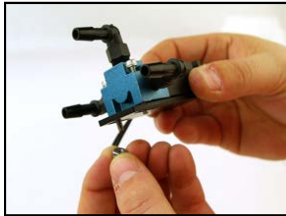
HDTCV being mounted to the bracket.
