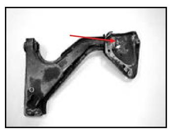
9 Separate the pocket bushing bracket from the lower control arm.
