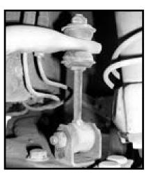
Remove the three 14mm bolts from the rear pocket bushing bracket.
