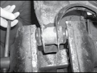
Begin assembling the pocket bushing bracket and lower control arm. Slide the bracket over the threaded rod on the control arm and be sure to use the included cup washer, beveled side toward the bushing, and the original washer and tighten the nut to 41 ft lbs.
