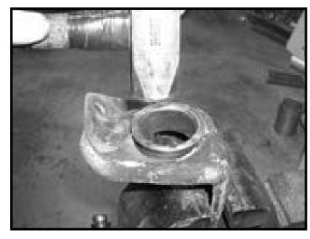
Using a small amount of the supplied grease install the new pocket bushing into the bracket/ sleeve assembly.
