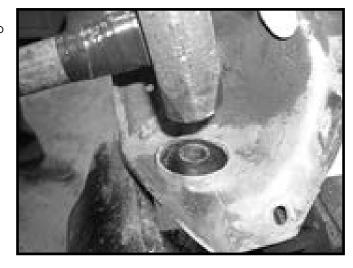
Install the supplied pocket bushing sleeve into its' bracket. Note the beveled edge in the bracket, install the new sleeve into this side. Hold the bracket in a vise and using a hammer with light to moderate force, knock the sleeve until it is fully seated into the bracket.
