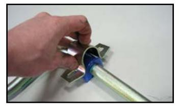
Install the four remaining original bolts and corresponding "D" shaped washers into the sway bar (saddle) mounting brackets. Tighten to 20 ft.lbs.
