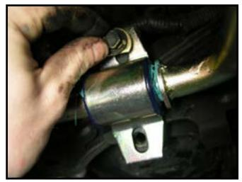
This bar kit is designed to fit two different control arm styles and it is easiest to tell them apart by the style of factory end-link which was installed. The shorter (pin/bolt style) is replaced using the shorter included bolts and sleeves. The longer (ball end style) is replaced using the longer included bolts and sleeves. Assemble and install the new end-links as illustrated and tighten the locknut until the grommets are just starting to bulge.
