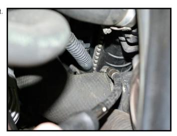
6 Remove the top engine boost pipe from the car.
