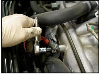
Now loosen the lower 7mm clamp at the turbo outlet.
