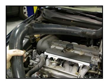
Remove the remaining 7mm clamps from the pipe and remove the old rubber couplers.
