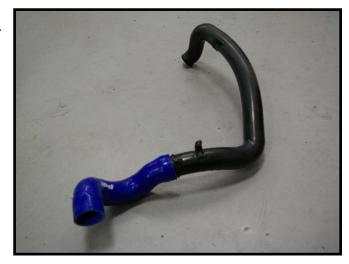
Reinstall the top engine boost pipe back into the vehicle with the new couplers installed on each end.
