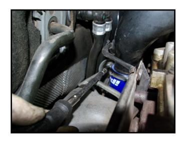
13 Reinstall the two torx 25 fasteners as shown.
