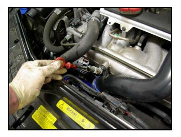
3 Begin by loosening the two torx 25 fasteners as shown.
