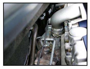
Now loosen the 7mm clamp at the intercooler inlet.
