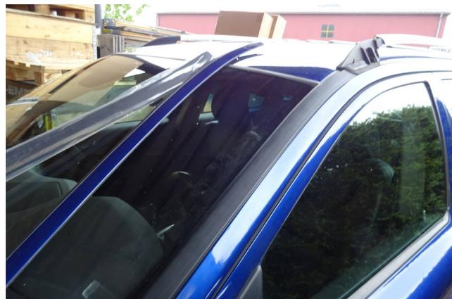
When the clips are all in place, slide the new moulding onto the top two clips and then snap it into place by pressing from above next to the windscreen.
