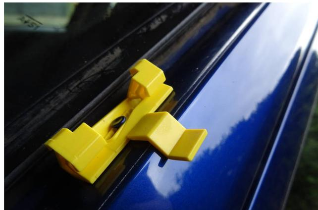
The three clips next to the windscreen (Skandix 1017092) have a depth stop to adjust the height of the clip on the body edge next to the windscreen frame.
