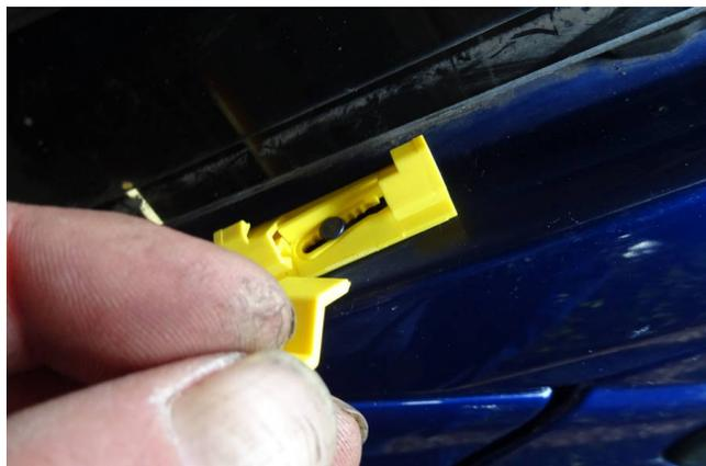
The depth stop is then broken off at the breaking point.
