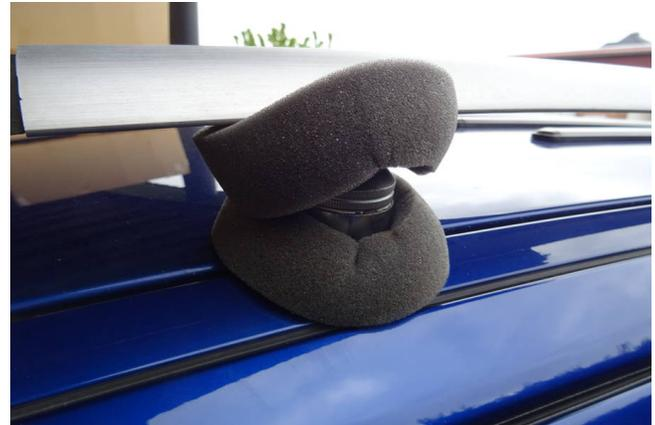
Lift the railing at the front and support it with something suitable so that the foot hangs approx. 2cm in the air.
