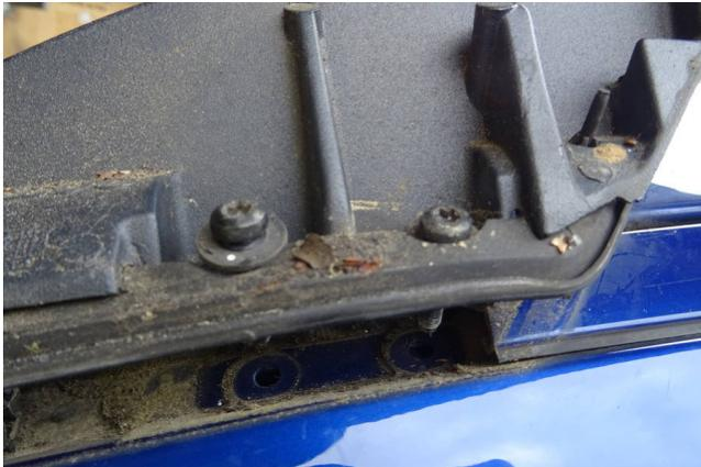
Loosen the two T30 screws of the rails completely.
