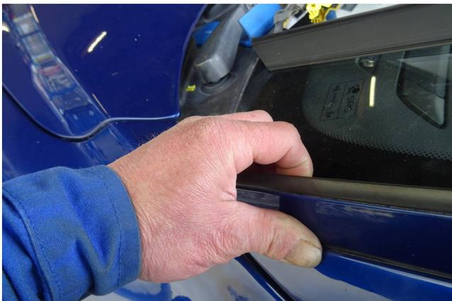
Now release the moulding from the lower three clips by folding it sideways outwards.
